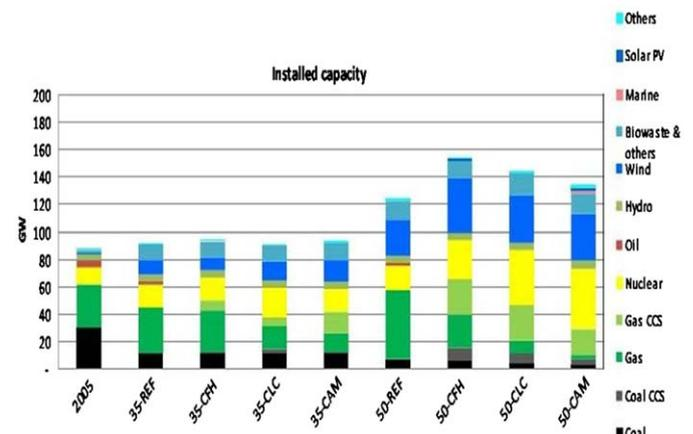
Fig. 7. Installed electric capacity (GW) for the different scenarios for years 2005, 2035 and 2050.
